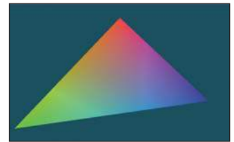
Figure 15.6: The single triangle scene visualized with color equal to barycentric weight for debugging the intersection code.
